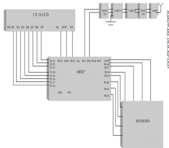
Figure:5 Hardware description of ARM with LCD and GSM module
