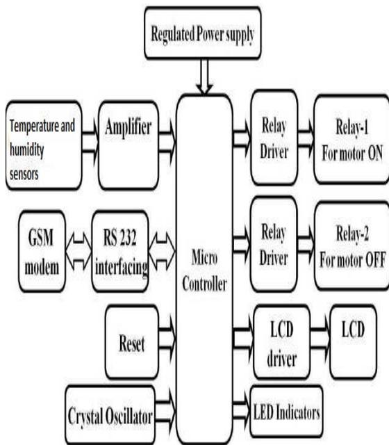
Figure –6 Block diagram of base station showing relays
