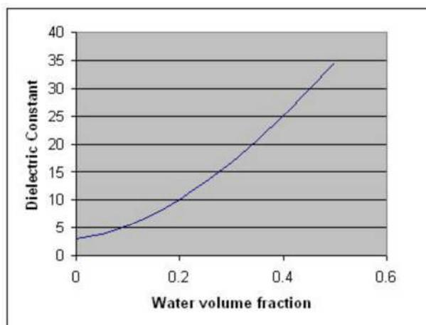
Figure.1 Dependence of Dielectric Constant of a Mixture on Water Content
