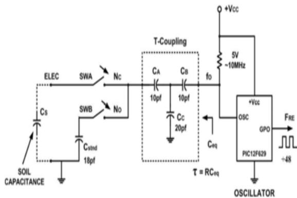
Figure-2 Frequency Shift Oscillator Circuit with Capacitance T-coupling Network
