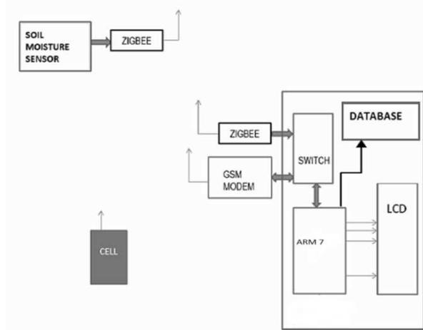
Figure :4 Centralized Base station Block Diagram
